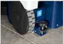
The idle wheel, placed near the rear driven wheel, allows the machine to be manually moved even without batteries.
