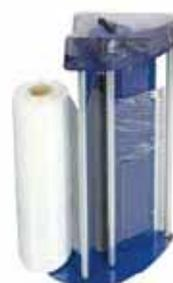
Carriage with mechanical brake on return roller, constant film elongations regardless spool diameter. Quick brake on/off device to facilitate film hooking to the base of the pallet. The brake intervenes on the rubber roller to allow wrapping tension adjustment. The extra metal rollers are positioned as to ensure a greater film embrace around the braking roller.
