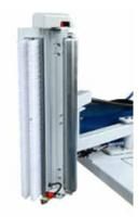
The innovative clamp and cut unit is based on a pneumatic system and delivers high precision and reliable performances by executing each operation step by step. The integrated spreading unit on the CS machines is able to spead the film at the end of each wrapping cycle and ensures the absence of any tail.
