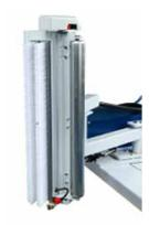
The innovative clamp and cut unit is based on a pneumatic system and delivers high precision and reliable performances by executing each operation step by step. The integrated spreading unit on the CS machines is able to spead the film at the end of each wrapping cycle and ensures the absence of any tail.
