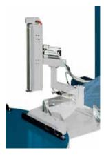
The innovative clamp and cut unit is based on a pneumatic system and delivers high precision and reliable performances by executing each operation step by step. The integrated spreading unit on the CS machines is able to spead the film at the end of each wrapping cycle and ensures the absence of any tail. The
