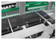
After the collation of the products into the required configuration, the block of the products is transferred to couple with the tray
