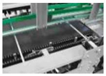
After the collation of the products into the required configuration, the block of the products is transferred to couple with the
