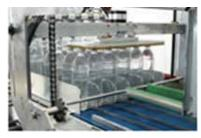
Control by means of photocells for correct product position and for minimum product accumulation in each channel. The product is separated in the
